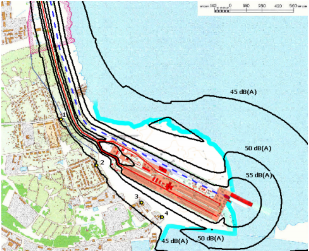
Figure 4.4 Noise impact from terminal operation activities including trains, vehicles and ferries, 3-shift working.
