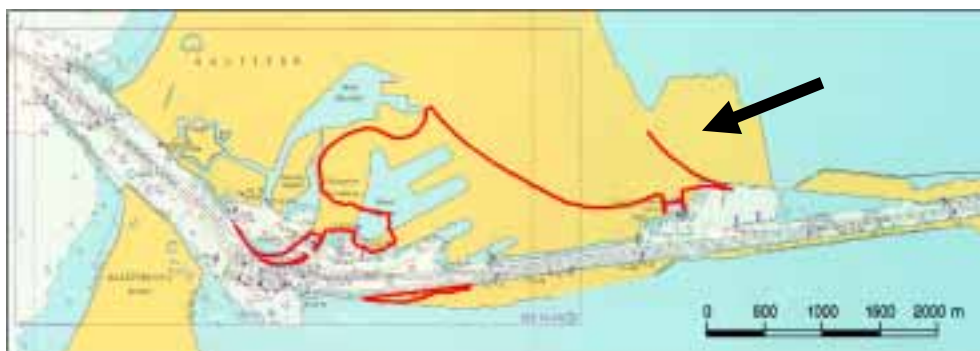
Figure 3.2 Illustration of the fact that the Vostochny peninsula (arrow) is younger than 1902. The coastline from a survey in 1902 (red line) is drawn on top of an Admiralty sea chart.
