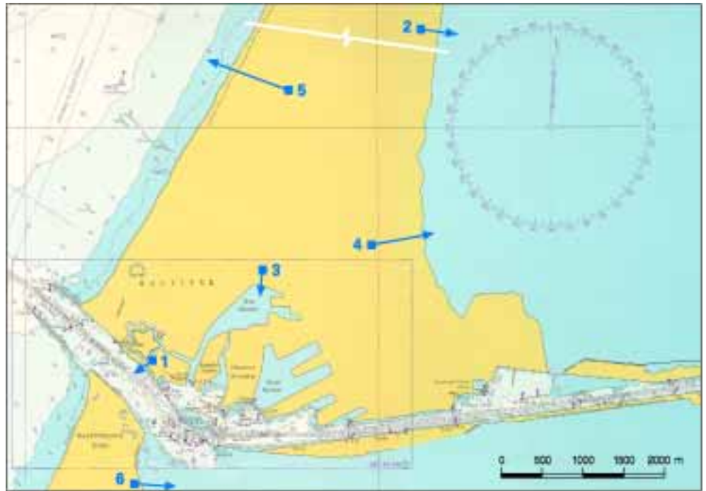
Figure 3.21 Illustration of the sewage discharges from Baltiysk to the marine environment. Discharge no.5 accounts for approximately half of the total discharge and the only discharge of treated sewage.
